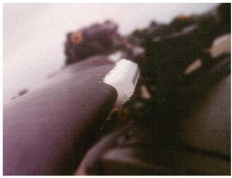
Approx 2 inches of ice on a leading edge. Not much in fixed wing terms but remember the size of the helicopter's 'wing' (rotor blade).
